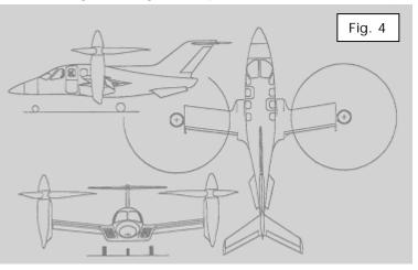
office as well. This twin, as configured here, can carry eight people, however, the propulsion concept of this patent can scale to quite large aircraft. It will need some extra space due to its two rotors being out on the wing tips. The one shown here has 19 foot rotors on a wing span of approximately 30 ft. This creates an overall of approximately 49 ft. The aircraft of Fig. 5 is shown in forward flight mode. This 8 place, 7,650 lb aircraft has been calculated to cruise at 385 mph at sea level.
