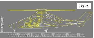
pilot would slowly begin diverting some of the exhaust to the main exhaust nozzle in the rear of the aircraft. Eventually, only enough exhaust would be diverted to the rotor to maintain its stability at about 150 rpm.
