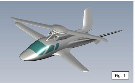
to sustain the aircraft above 115 mph; therefore, their reduced size (compared to typical fixed wing aircraft) significantly decreases drag and improves performance. Once flying on the wings, the rotor is no longer needed so it is slowed down to, again, reduce drag.
